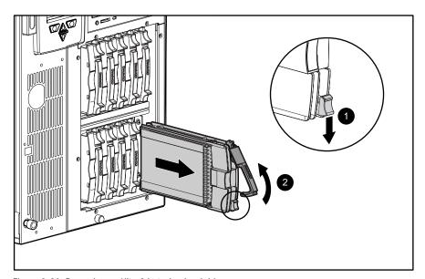
Figure 2-20. Removing an Ultra2 hot-plug hard drive
